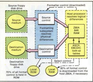
Fig. 3. The translation process between two floppy disks begins with the formatting subsystem reading the file directory information from the source medium. Formatter control information is downloaded from the host. Source records are buffered and manipulated in the Z80A under control of BASIC translation programs. Records are then written to the destination medium via the formatting subsystem according to physical requirements.
