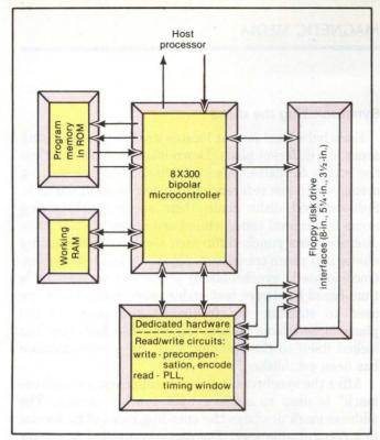
Control files down-loaded to the microcontroller's RAM evoke subroutines stored in ROM. About 70 percent of all formatting control is held in this firmware; the balance is down-loaded from the host's BASIC program when needed and is executed directly from RAM (Fig. 3).
