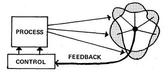
As an example, our engine driver will note the divergence of his measured speed from the objective and adjust the throttle in such a way as to reduce this deviation. The point about having a closed loop control is that it does not matter what disturbance occurs, perhaps a slight change in the output such as the engine going up an incline; but the deviation from objective is immediately spotted and the appropriate corrective action taken.
