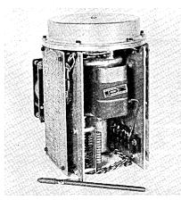
The new memory systems have 8 data tracks with 18,125 bits per track. Average access time is 8.5 milliseconds. The 8100 series may be used as the main storage on electronic calculators and small computers, as a replacement for delay line memories, as a buffer memory or as a data storage device on special purpose digital systems. (For more information, circle #48 on the Reader Service Card.)
