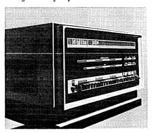
Initially the PDP-11 will be offered in two models: a special purpose controller, the PDP-11/10, equipped with central processor, 1024 words of read-only memory, and 128 words of standard memory; and the PDP-11/20, a general purpose computer with central processor, 4096 words of standard core memory expandable to 32,768 words, a programmer's control panel, and Teletype.
