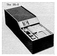
The DS-80 reader is complete and self-contained with interface, modular circuitry, and performance features that are compatible with most computers and data systems. It reads Hollerith coded data on command, a column at a time, up to speeds of 80 columns a second. Features include single-step function with return to start from any column; automatic feed and return; sync/output with read control; and 3 speeds determined by application. All control functions are remotely programmed.
