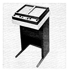
Operator-oriented controls are all positioned on the front panel. Plot sizes up to 10" x 15" are continuously adjustable through an "absolute plot dimension" pushbutton facility. Plotting speed is 150 to 225 points per minute depending upon the particular system used.
