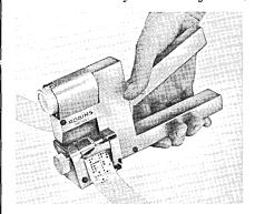
A selector knob in the front of the device permits quick and easy selection of the code desired. An indicator window at the top front shows the exact character being punched. After each code is made, the tape is automatically fed to the next punching position. (For more information, circle 54 on the Readers Service Card.)
