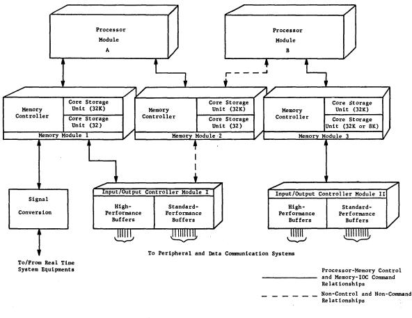
Figure 2. Typical Multicomputer Configuration of a GE-600 Computer
