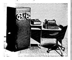
The machine is compatible with any input-output keyboard or tape typewriter chosen by the user. It will accept and produce 5, 6, 7, or  $\vartheta$  channel tape up to 1 inch wide, in any tape code. Tapes are processed at rates of 500 words per minute. The new machine has application in all areas where perforated tape is used, and particularly in data preparation for computers. (For more information, circle 52 on the Readers Service Card.)
