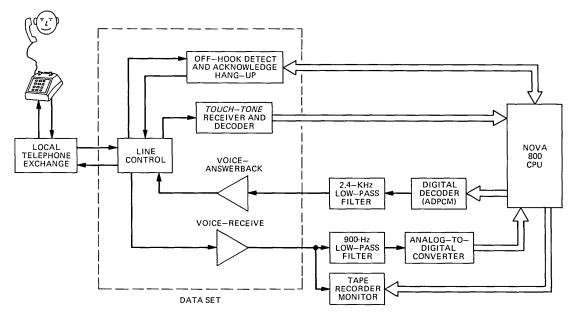
Fig. 4—Experimental setup block diagram showing the principal components of apparatus linking the customer's telephone and the computer.
