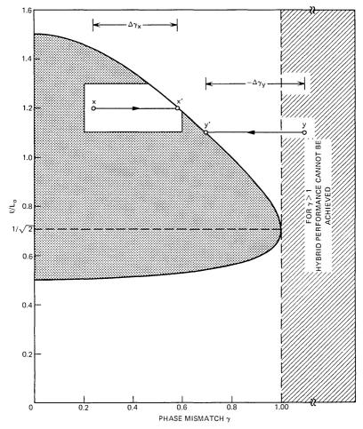
Fig. 2—Required coupler length  $(l/L_0)$  to obtain hybrid operation as a function of the phase mismatch parameter  $\gamma$  of the coupler.
