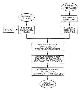
Fig. 1—System-operation block diagram.
