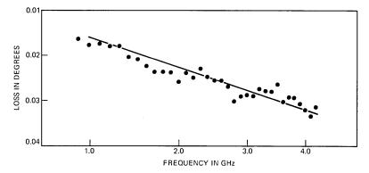
Fig. 13—S21 phase of a 50-ohm airline.
