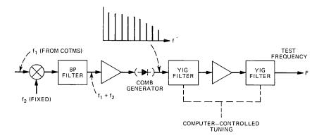
1-4 GHz MEASURING SET :  $f_2$  = 198 MHz, 22 MHz  $\leqslant$   $f_1 \leqslant$  77 MHz 4-12 GHz MEASURING SET :  $f_2$  = 825 MHz, 75 MHz  $\leqslant$   $f_1 \leqslant$  300 MHz
