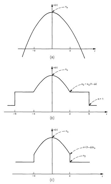
Fig. 1—(a) Ideal parabolic-index profile of eq. (3). (b) Truncated parabolic-index profile of eq. (4). This profile is used for mode filters. (c) Modified parabolic-index profile of eq. (5). This profile is used for the fiber with intentional mode coupling.
