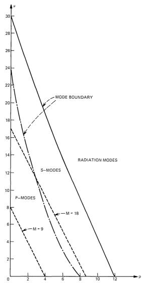
Fig. 2—Mode number space. The solid line is the boundary between S-modes and radiation modes. The dash-dotted line is the boundary between S-modes and P-modes. The dotted lines labeled M=9 and M=18 are curves of constant compound mode number M. M=18 is used as approximate mode boundary.
