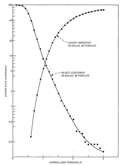
Fig. 7—Error rate vs normalized threshold. The effects are given of threshold variation on the reject-customer and accept-impostor rates using the operational accept/reject criterion.
