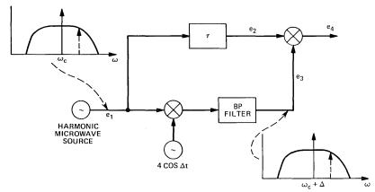
Fig. 6—Second-order noise product mechanism.
