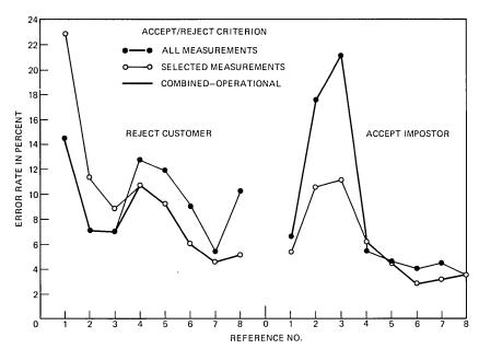
Fig. 6—Average error rates vs reference update. Reject-customer rates are plotted on the left and accept-impostor rates on the right. The thick line in each case shows the error rate under the operational criterion.
