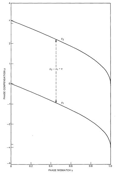
Fig. 3— $\phi_1$  and  $\phi_2$  required to switch on State I and II, respectively, assuming identical coupler pairs and both being adjusted to provide hybrid operation.
