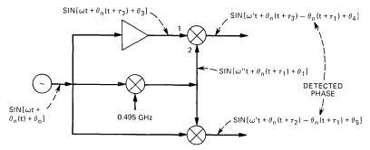
Fig. 5-Phase-noise cancellation mechanism.
