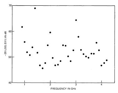
Fig. 15—S11 magnitude of a 50-ohm airline.
