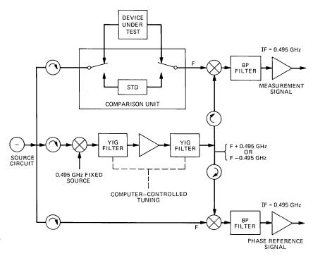
Fig. 3—Block diagram of the heterodyne circuitry.
