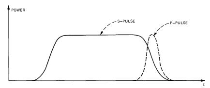
Fig. 4—The solid line is the shape of the S-pulse that results from coupling of P-mode power whose shape is indicated by the dotted line. The relative height of the two pulses is of no significance.
