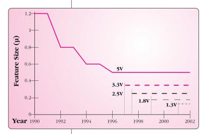
Rapidly shrinking device geometries will require the use of smaller supply voltages.
