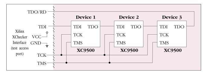
and then shifting out the result, you can effectively and automatically test devices and their interconnections on a PC board.
