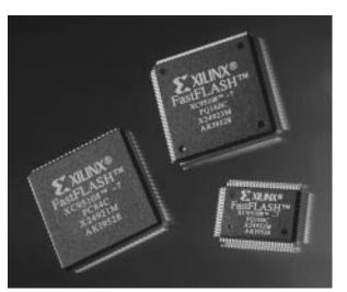
The powerful XC9500 architecture supports a wide variety of design methodologies. Each function block and macrocell is identical. This assists the designer when using HDLs, synthesis and/or schematic capture tools by
