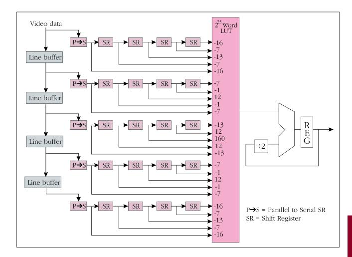
Consequently, serial adders can be used to combine four serial bit streams into one before addressing the multiplying LUT (Figure 3). Effectively, this adds, and then weights, data that would otherwise be weighted and added afterwards. A tree of three serial adders is needed in each case, and each serial adder can be implemented in a single CLB.
