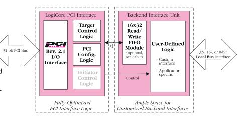
programmable gates remain free for integration of the unique, back-end functions of the application. This is a high-performance, one-chip solution.
