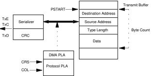
Figure 5. Packet Transmission
