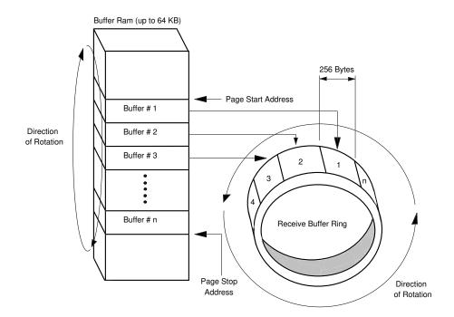
Figure 7. Receive Buffer Ring
