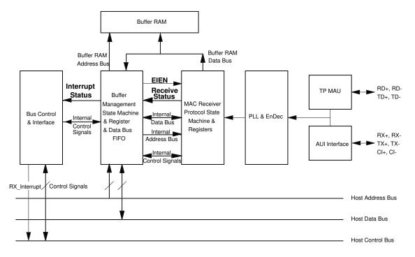
*Figure 12: Early Interrupt Receive Block Diagram* **12.1. Early Interrupt Architecture Programming Algorithm**
