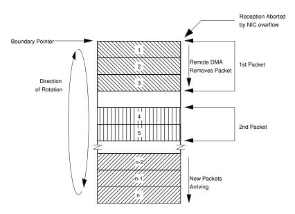
Figure 11. Receive Buffer Ring Overwrite Protection
