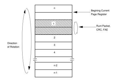
Figure 9. Packet Rejection
