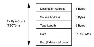
Figure 4. Transmit Packet Format
