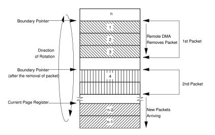
Figure 10. Removing Packets from the Receive Buffer Ring
