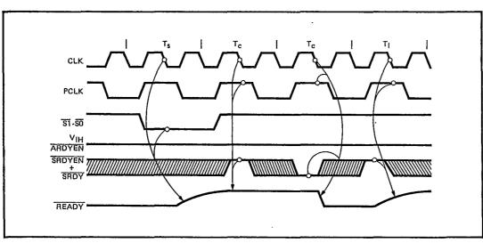
Figure 3. Synchronous Ready Operation
