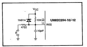
Figure 2. Typical RC RES Timing Circuit
