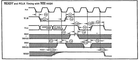
Note 1: This is an asynchronous input. The setup and hold times shown are required to guarantee the response shown. Note 2: Tie 700 ohm  $\pm 5\%$  pullup resistor to the READY output.
