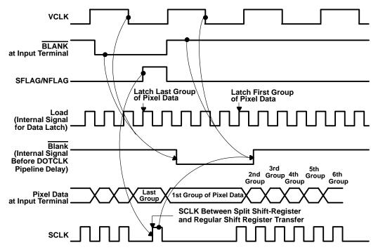
NOTE A: Either the SSRT function is disabled (general-control register bit 2 = 0), or the SFLAG/NFLAG input is held low when the SSRT function is enabled (general-control register bit 2 = 1).
