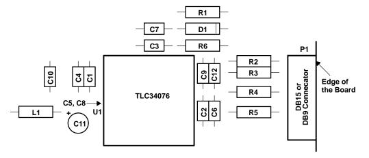
Figure B-2. Typical Component Placement (Component Side)
