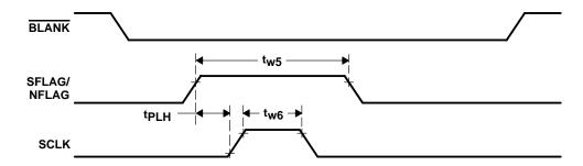
Figure 3–3. SFLAG/NFLAG Timing (When SSRT Function is Enabled)
