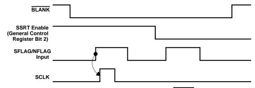
Figure 2-9. Relationship Between SFLAG/NFLAG, BLANK, and SCLK
