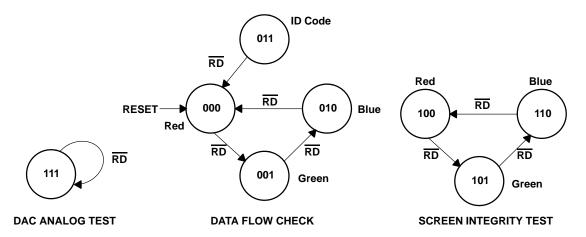
Figure 2-11. Test-Register Control-Word State Diagrams
