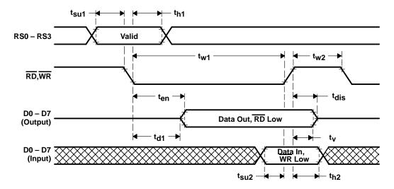
Figure 3–1. MPU Interface Timing
