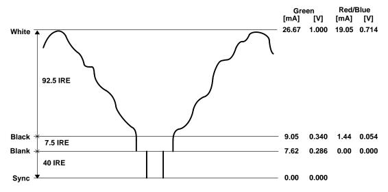
Figure 2-7. 7.5-IRE, 8-Bit Composite Video Output
