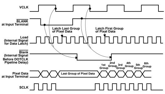
Figure 2–4. SCLK/VCLK Control Timing (SSRT Disabled, SCLK Frequency = 4 × VCLK Frequency)
