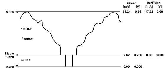
Figure 2-8. 0-IRE, 8-Bit Composite Video Output
