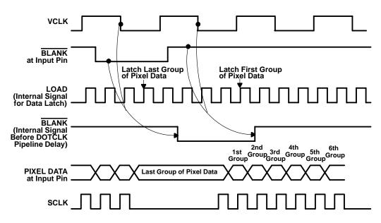
Figure 6. SCLK/VCLK Control Timing (SSRT Disabled, SCLK Frequency = 4 × VCLK Frequency)
