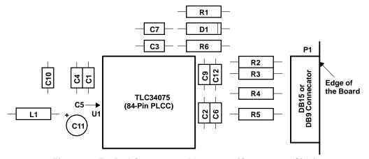
Figure 19. Typical Component Placement (Component Side)
