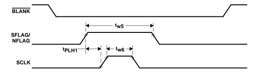
Figure 17. SFLAG/NFLAG Timing (When SSRT Function is Enabled)
