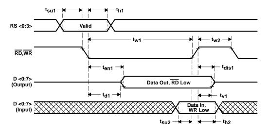
Figure 15. MPU Interface Timing
