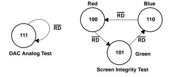
Figure 13. Test Register Control Word State Diagrams
