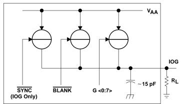
Figure 8. Equivalent Circuit of the IOG Current Output
