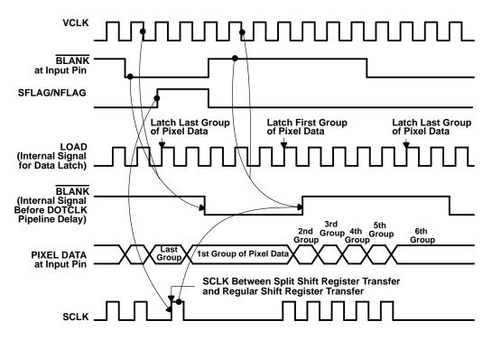
NOTE: The SSRT function is enabled (general control register bit 2 = 1).
