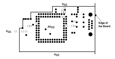
Figure 20. Typical Split Power Plane (Solder Side)
