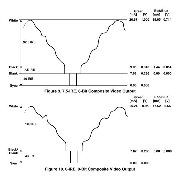
NOTE: 75- $\Omega$  doubly terminated load. V<sub>REF</sub> = 1.235 V, R<sub>SET</sub> = 523  $\Omega$ . RS-343A levels and tolerances are assumed.
