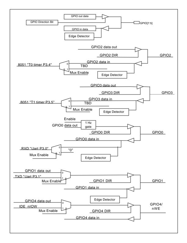
FIGURE 2 - GPIO MUXING BLOCK DIAGRAM
