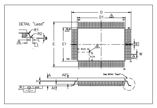
FIGURE 7 - 100 PIN QFP PACKAGE
