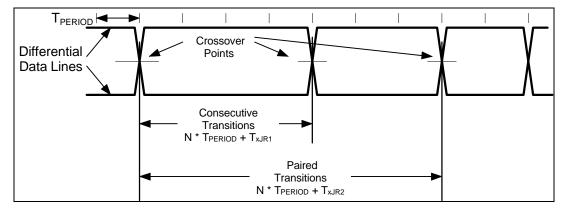
FIGURE 7 - DIFFERENTIAL DATA JITTER
