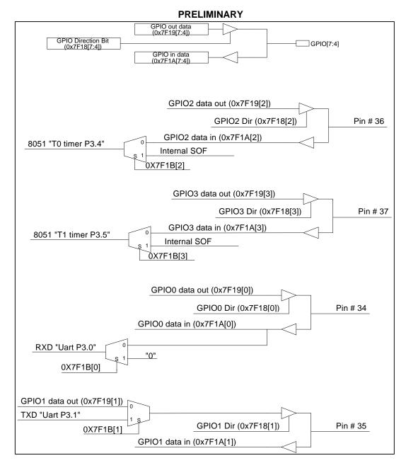
FIGURE 3 - GPIO MUXING BLOCK DIAGRAM
