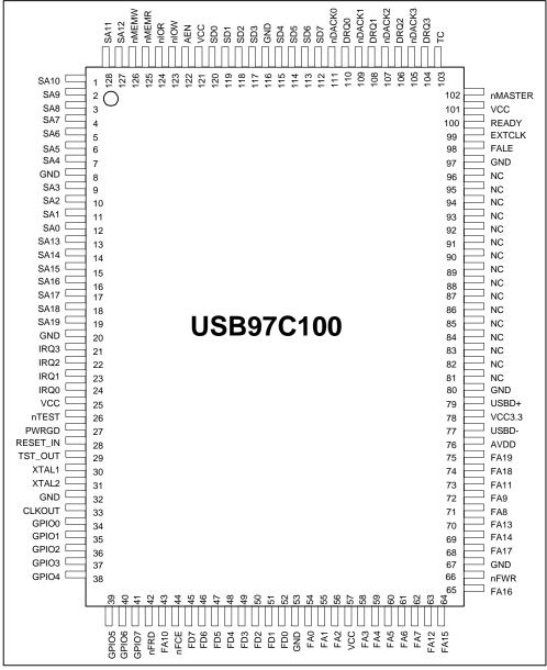
**FIGURE 1 - PIN CONFIGURATION**
