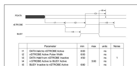
1. The data is held until BUSY goes inactive or for time t3, which ever is longer. This only applies if another data transfer is pending. If no other data transfer is pending, the data is held indefinitely.
