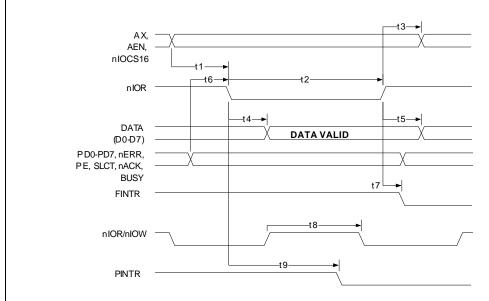
NOTE: PINTR is the interrupt assigned to the Parallel Port FINTR is the interrupt assigned to the Floppy Disk
