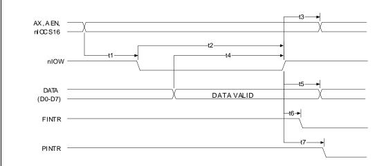
NOTE: PINTR is the interrupt assigned to the Parallel Port FINTR is the interrupt assigned to the Floppy Disk
