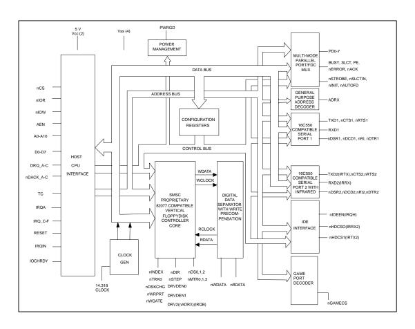
FIGURE 1 - FDC37C669 BLOCK DIAGRAM
