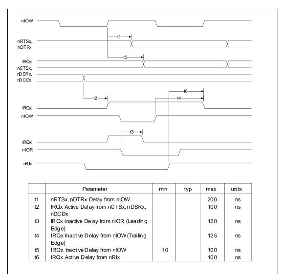
FIGURE 8 - SERIAL PORT TIMING
