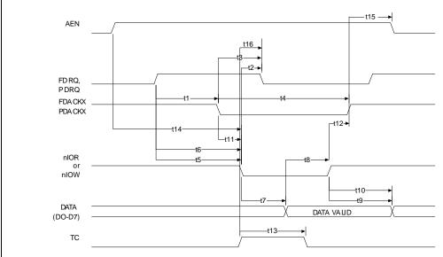
NOTE: FDRQ refers to the DRQ assigned to the Floppy Disk PDRQ refers to the DRQ assigned to the Parall el Port FDACKX refers to the DRQ assigned to the to the Floppy Disk PDACKX refers to the DRQ assigned to the Parallel Port
