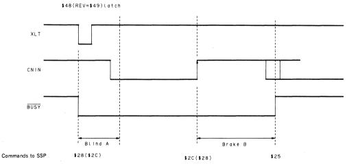
Figure 3-9 (b) Timing chart for 1-track jump
