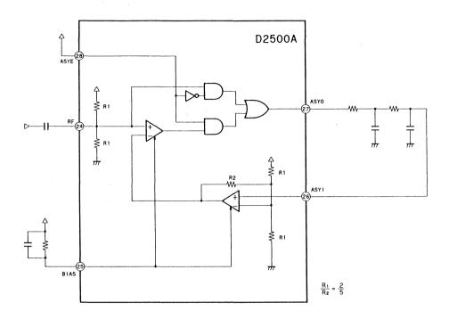
Figure 3-15 Asymmetry correction application circuit example
