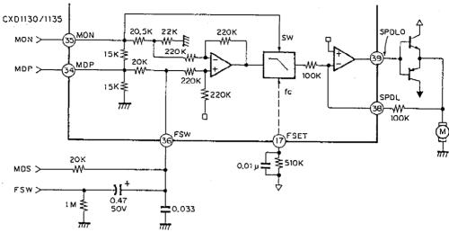
The 200 Hz LPF is formed with 0.033  $\mu$ F and 20 k $\Omega$  connected to pin 36. The secondary LPF is formed with the built-in LPF (fc up to 200 Hz with 510 k $\Omega$  for pin 17), and the carrier component of the CLV servo error signals MDS and MDP is eliminated.
