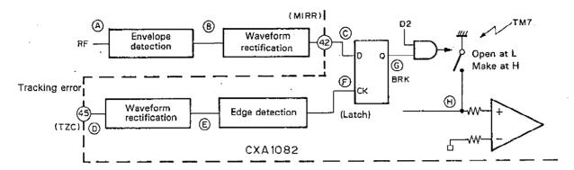
Fig. 6 TM7 Movement (Break Circuit)
