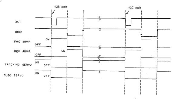
2. LOCK (Sled runaway prevention circuit)
