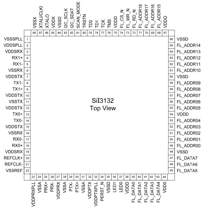
Figure 1. Pin Diagram (Top View)
