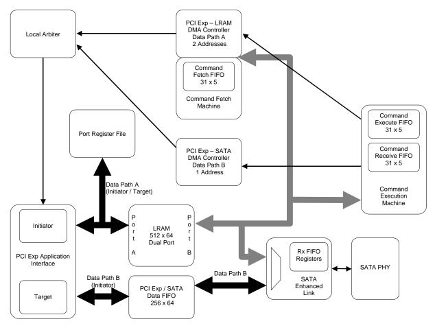
Figure 6. Port Logic Block Diagram
