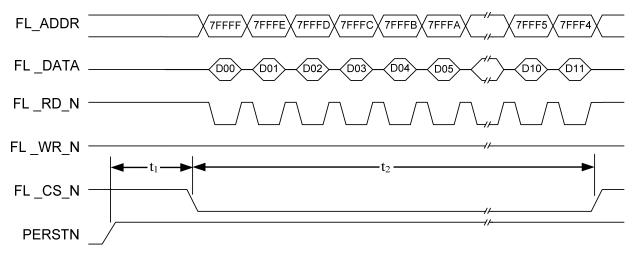
Figure 8. Auto-Initialization from Flash Timing
