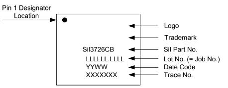
Figure 10: Marking Specification - Sil3726CB
