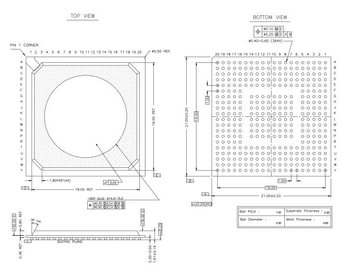
Figure 9: 364 Ball HSBGA Package Dimensions (in Millimeters)
