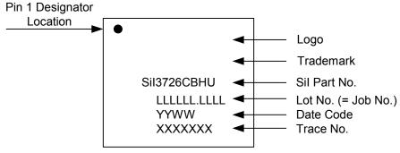
Figure 11: Marking Specification - Sil3726CBHU
