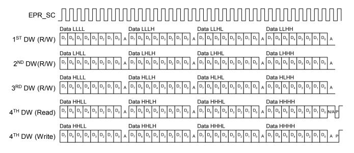
Figure 5: I<sup>2</sup>C Block Transfer
