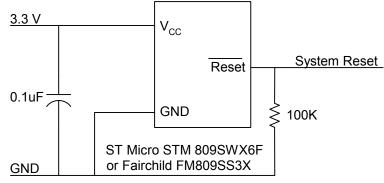
Figure 6: Power-Up Reset Circuit
