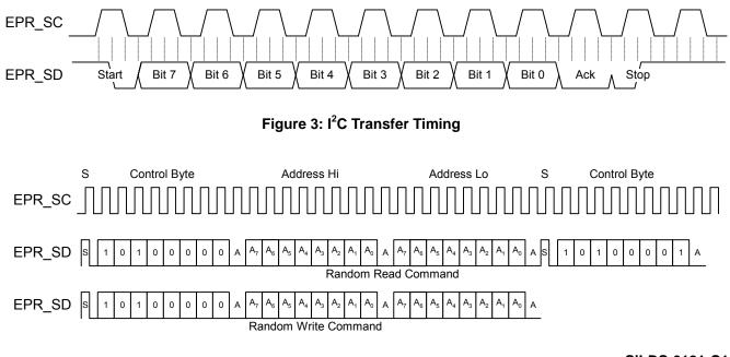
Figure 4: I<sup>2</sup>C Random Read and Write Timing
