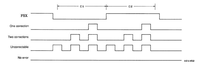
The 7.35 kHz FSX frame synchronization signal is divided down from the reference clock. The status of error correction in each frame is output on EFLG, as shown in the figure, where the number of high pulses in each FSX period indicates the quality of the replay signal.
