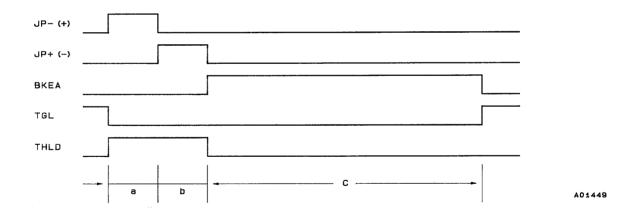
When a track jump command is issued to the servocontroller, an acceleration pulse is generated (a period), followed by a deceleration pulse (b period) and braking (c period), completing the specified jump. TES and HFL input during braking detects the direction of beam slippage, and the portion of the TE signal that compensates for slippage is cut off by TOFF, which, together with boosting of the servo gain by TGL, supplements the destination track for the jump.
