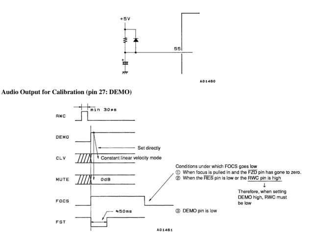
Setting this pin high sets muting to 0 dB and the disc motor to constant linear velocity, even when the microprocessor issues no command, and activates focusing. Because this also makes the  $\overrightarrow{LASER}$  pin active, EFM signals and audio output can be obtained without the microprocessor as long as the mechanism and servo are hooked up correctly.
