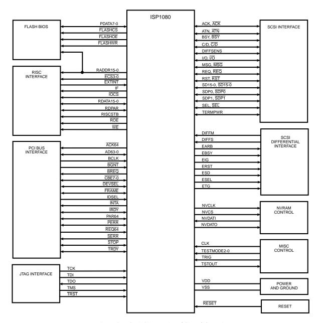
Figure 3. ISP1080 Functional Signal Grouping
