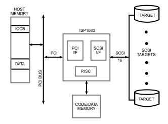
Figure 2. I/O Subsystem Design Using the ISP1080
