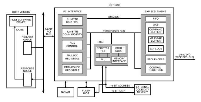
Figure 1. ISP1080 Block Diagram
