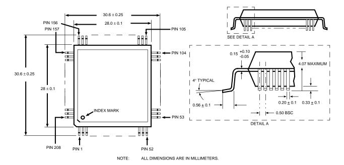
Figure 4. ISP1040B Mechanical Drawings
