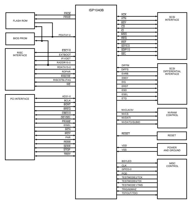
Figure 3. ISP1040B Functional Signal Grouping
