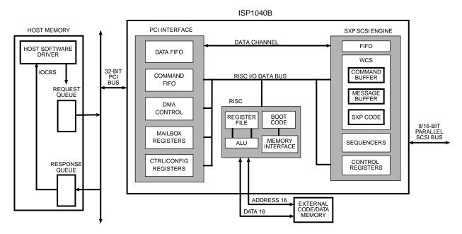
Figure 1. ISP1040B Block Diagram
