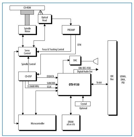
Block Diagram of CD-ROM Drive Electronics
