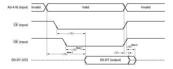
Notes 1. To read within the range of tacc (< 118 >), the delay time of  $\overline{OE}$  input from the falling of  $\overline{CE}$  must be tacc-toe (< 118 > - < 120 >) max.
