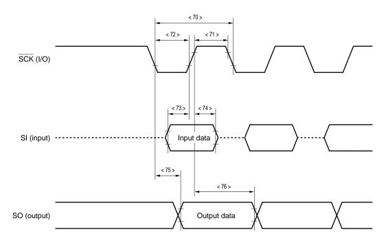
**Remark** The broken line indicates the high-impedance state.
