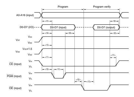
Cautions 1. Apply VDD before VPP, and turn off VDD after VPP.
