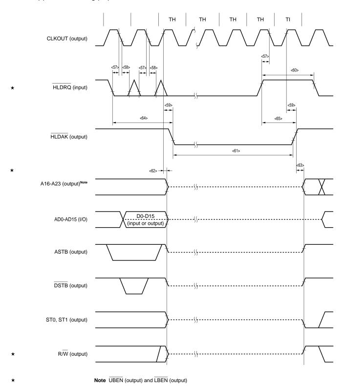
Remark The broken line indicates the high-impedance state.
