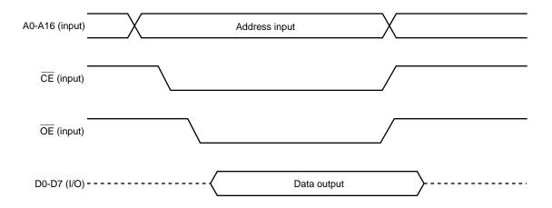
Remark The broken line indicates the high-impedance state.
