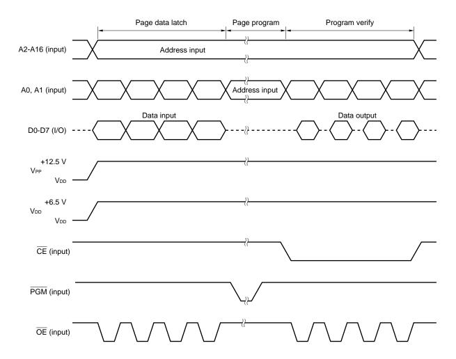
**Remark** The broken line indicates the high-impedance state.
