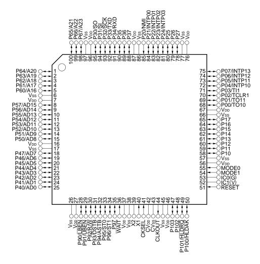
Caution The letters in brackets ( ) indicate the processing of the pins not used in the normal operation mode.
