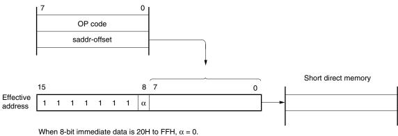
When 8-bit immediate data is 20H to FFH,  $\alpha = 0$ . When 8-bit immediate data is 00H to 1FH,  $\alpha = 1$ .
