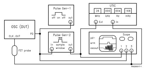
FIGURE 1. Sample Measurement Setup
