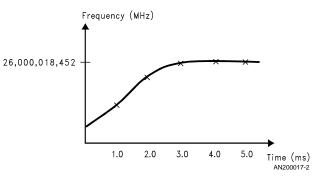
FIGURE 2. Plot of a Xtal Oscillator Startup Time Profile
