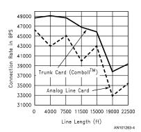
FIGURE 4. Average Connection Rates vs Line Length (V.90 Modem B with AWG 26)
