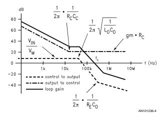
FIGURE 4. Bode Plots of Transfer Functions
