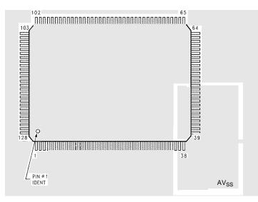
Figure 5. AV<sub>SS</sub> Plane Layout Example
