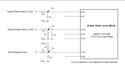
Figure 2. Analog Input Examples
