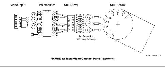
After the parts are placed, the trace routing should be done using a prioritized list with the HF signals, power and ground at the top of the list. Following should be the low frequency signals and then finally any DC signals. Attention must also be paid to avoid coupling the HF signals unto the low frequency signal traces (crosstalk). Crosstalk will be discussed later in this article.
