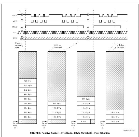
After the preamble and the SFD (Point A), the FIFO shifts in  $74\pm1$  bit of data (depending on the location of the SFD with respect to t1 of the DMA sequence) before BREQ is asserted (Point B). The FIFO transfers 2 bursts of 4 bytes each into memory while shifting in 23 bits of data until
