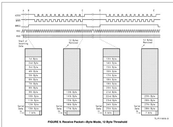
After the preamble and the SFD (Point A), the FIFO shifts in  $111\pm 2$  bits of data (depending on the location of the SFD with respect to t1 of the DMA sequence) before BREQ is asserted (Point B). The FIFO transfers 1 burst of 12 bytes into memory while shifting in 26 bits of data until  $\overline{\rm MWR}$  is
