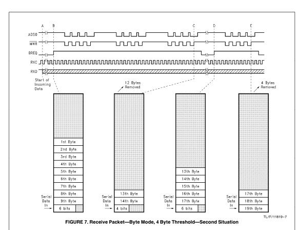
After the preamble and the SFD (Point A), the FIFO shifts in  $78\pm1$  bit of data (depending on the location of the SFD with respect to 11 of the DMA sequence) before BREQ is asserted (Point B). The FIFO transfers 3 bursts of 4 bytes each into memory while shifting in 38 bits of data until
