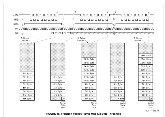
The FIFO prefetches 8 bytes from memory (Point A). The preamble starts during these prefetches. After the preamble and the Start of Frame Delimiter are transmitted, data is shifted out of the FIFO. After 22 bits are shifted out, BREQ is asserted (Point B). During this burst, 8 bytes are loaded
