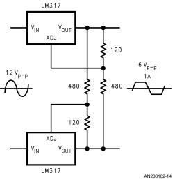
FIGURE 12. AC Voltage Regulator
