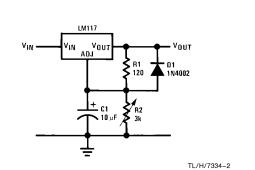
FIGURE 2. Basic Voltage Regulator
