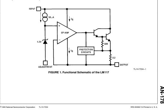
Applications for an Adjustable IC Power Regulator
