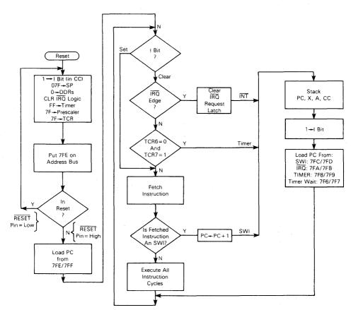
FIGURE 14 -- RESET AND INTERRUPT PROCESSING FLOWCHART
