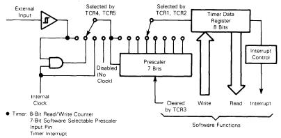
FIGURE 18 - PROGRAMMABLE TIMER/COUNTER BLOCK DIAGRAM
