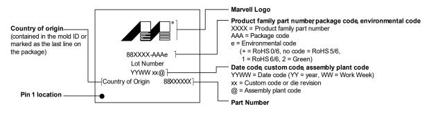
**Note:** The above drawing is not drawn to scale. The location of markings is approximate. Add-on marks are not represented. Flip chips vary widely in their markings and flip chip examples are not shown here. For flip chips, the markings may be omitted per customer requirement.
