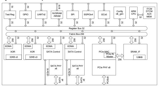
Figure 1-1 88SE1475 System Architecture
