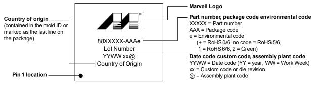
**Note:** The above drawing is not drawn to scale. The location of markings is approximate. Add-on marks are not represented. Flip chips vary widely in their markings and flip chip examples are not shown here. For flip chips, the markings may be omitted per customer requirement.
