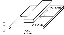
Figure 4-4 shows the thermal ground plane in relation to the return-path capacitor.
