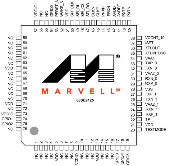
**Note:** The center area beneath the chip is the Exposed Die Pad (Epad). When designing the PCB, create a solder pad for the Epad and connect the Epad to ground.
