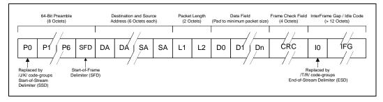
Figure 18. 100BASE-TX Data Path
