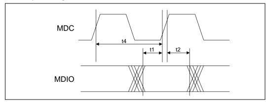
Figure 38. MDIO Output Timing
