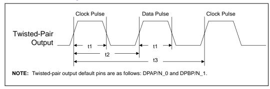
Figure 36. FLP Burst Timing
