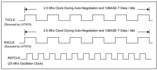
Figure 24. 100BASE-T DTE Mode Auto-Negotiation
