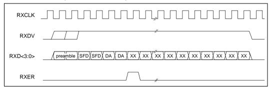
Figure 21. 100BASE-TX Transmission with no Errors
