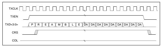
Figure 22. 100BASE-TX Transmission with Collision
