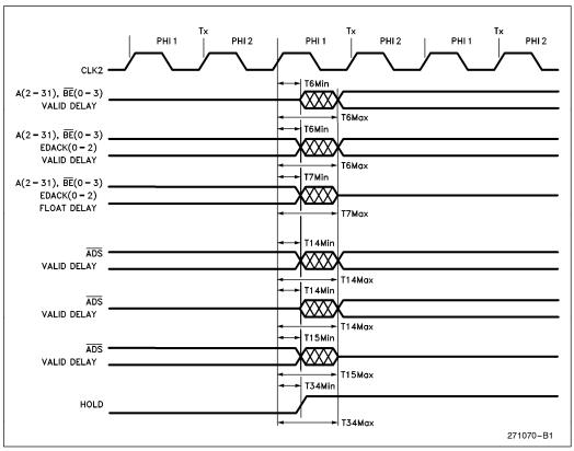
Figure 70. Address Output Delays
