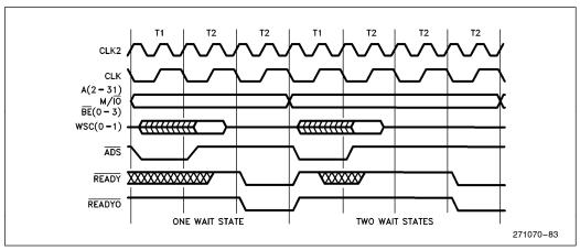
Figure 50. Wait States in Non-Pipelined Cycles
