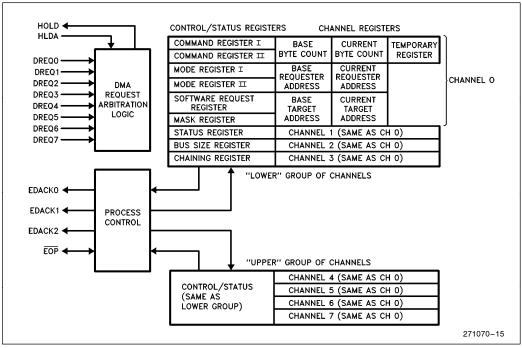
Figure 14. M82380 DMA Controller Block Diagram
