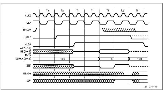
Figure 18. DMA Single Transfer Mode
