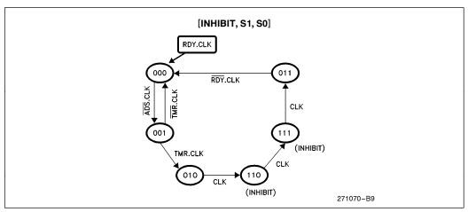
Figure 3. State Diagram for Inhibit Signal
