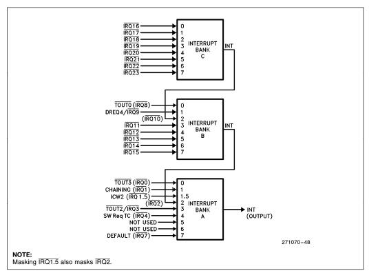
Figure 37. Interrupt Controller Block Diagram
