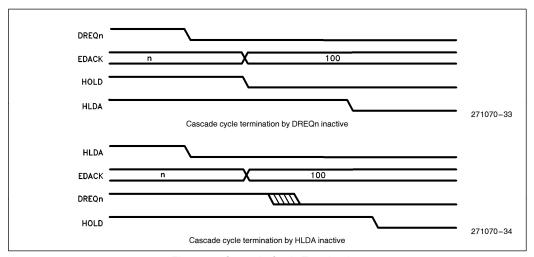
Figure 34. Cascade Cycle Termination
