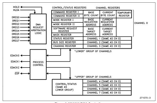
Figure 2. M82380 DMA Controller
