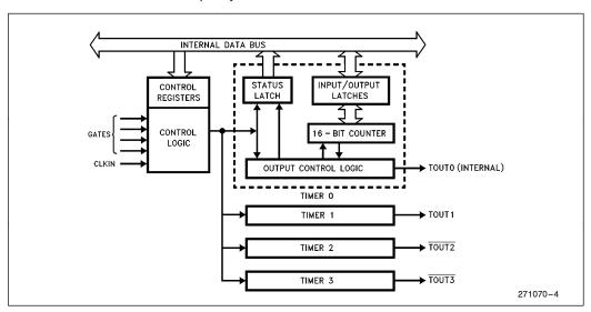
Figure 3. Programmable Interval Timers—Block Diagram
