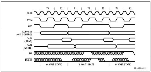
Figure 11. Non-Pipelined Bus Cycles
