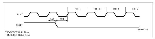
Figure 8. RESET Timing
