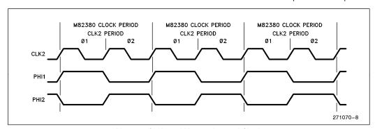
Figure 7. CLK2 and M82380 Internal Clock
