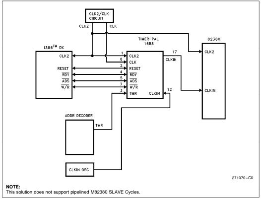
Figure 4. System with M82380 Timer Unit "Inhibit" Circuitry
