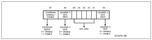
Figure 60. Internal Control Port
