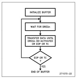
Figure 21. Buffer Transfer in Demand Transfer Mode
