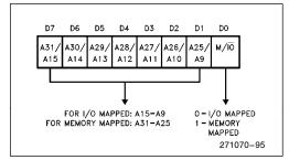
Figure 59. Relocation Register
