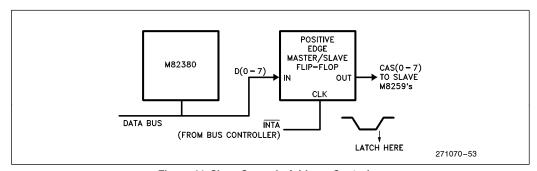
Figure 41. Slave Cascade Address Capturing
