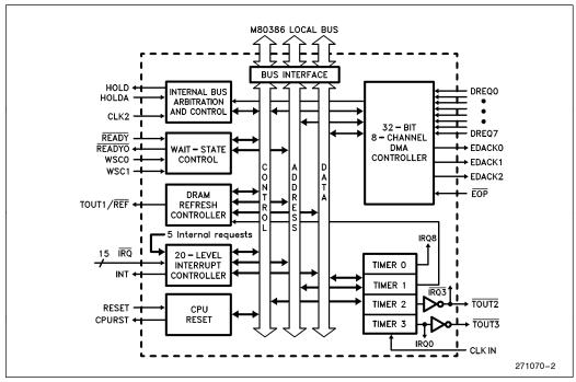
Figure 1. Architecture of the M82380
