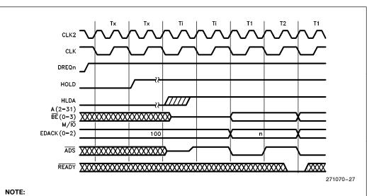
Channel priority resolution takes place during the bus state before HLDA is asserted, allowing the DMA Controller to respond to HLDA without extra idle bus states.
