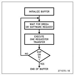
Figure 17. Buffer Transfer in Single Transfer Mode
