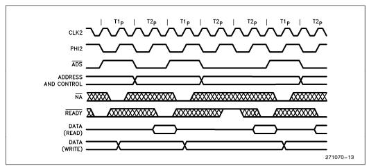
Figure 12. Pipelined Bus Cycles
