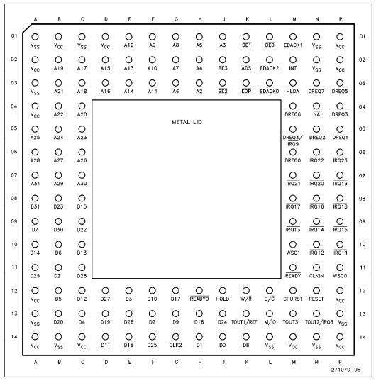
Figure 63. M82380 PGA Pinout—View from PIN side
