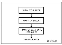
Figure 19. Buffer Transfer in Block Transfer Mode
