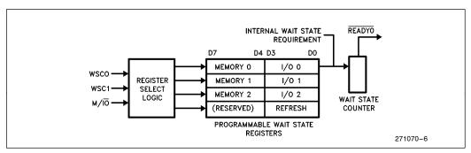
Figure 5. M82380 Wait State Generator—Block Diagram
