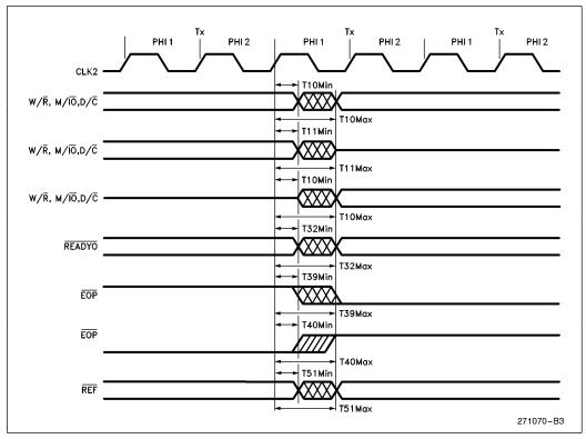
Figure 72. Control Output Delays
