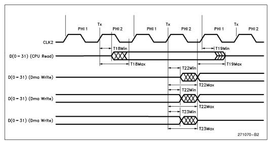
Figure 71. Data Bus Output Delays
