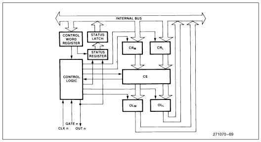
Figure 44. Internal Block Diagram of A Counter
