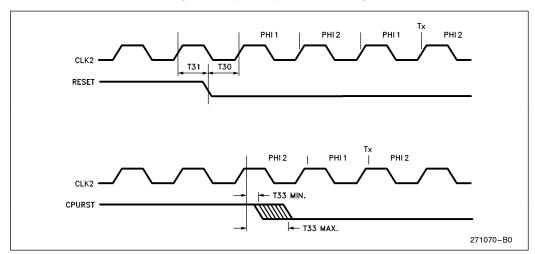
Figure 69. Reset Timing
