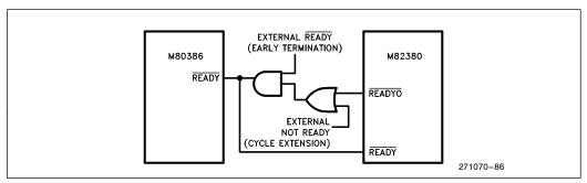
Figure 53. External 'READY' Control Logic
