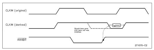
Figure 5(b). Inhibited CLKIN in an M82380 Timer Unit and CLKIN Minimum LOW Time
