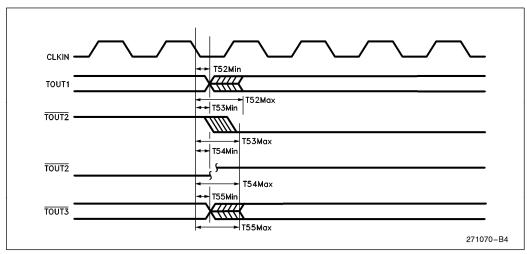
Figure 73. Timer Output Delays
