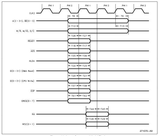
Figure 68. Input Setup and Hold Timing
