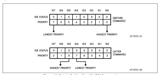
Figure 40. Rotate On Non-Specific EOI Command
