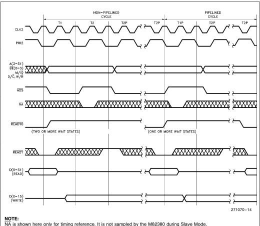
NA is shown here only for timing reference. It is not sampled by the M82380 during Slave Mode. When the M82380 registers are accessed, it will take one or more wait states in pipelined and two or more wait states in non-pipelined cycle to complete the internal access.
