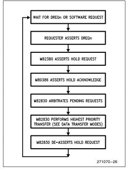
Figure 27. Bus Arbitration and DMA Sequence
