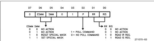
ESMM—Enable Special Mask Mode. When this bit is set to 1, it enables the SMM bit to set or reset the Special Mask Mode. When this bit is set to 0, SMM bit becomes don't care.
