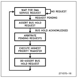
Figure 15. Flow of DMA Controller Operation
