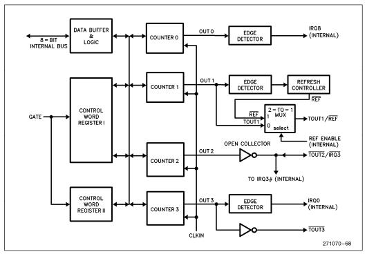
Figure 43. Block Diagram of Programmable Interval Timer
