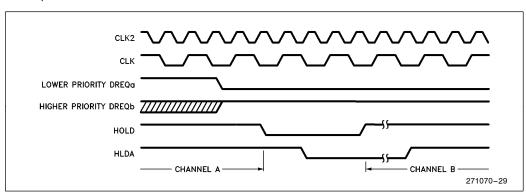
Figure 30. Switching between Active DMA Channels
