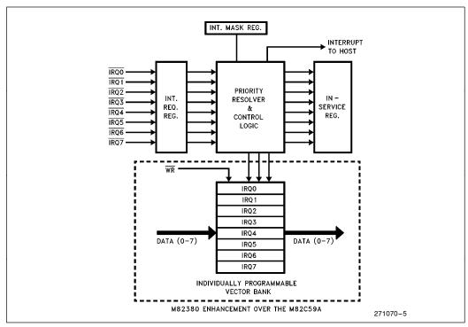
Figure 4. M82380 Interrupt Controller—Block Diagram
