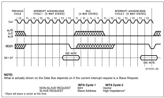
Figure 39. Interrupt Acknowledge Cycle
