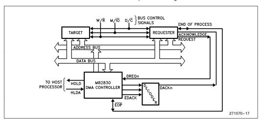
Figure 16. Requester, Target, and DMA Controller Interconnection
