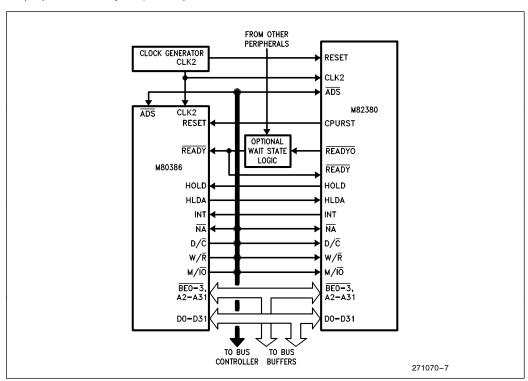
Figure 6. i386™/M82380 System Configuration
