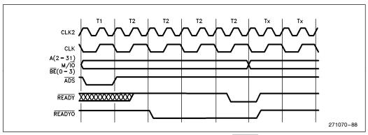
Figure 55. Extending Bus Cycle by 'READY'
