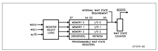
Figure 49. Wait State Generator Block Diagram
