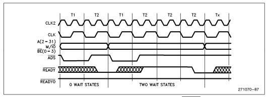
Figure 54. Early Termination of Bus Cycle by 'READY'
