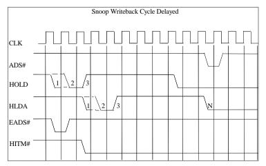
**IMPLICATION:** If the system expects a cycle, for example a writeback cycle, and depends on this cycle to commence within the HLDA deassertion window, then the system may not complete the handshake and cause a hang.
