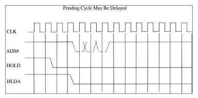
In two cases, for example, if HOLD is deasserted for one clock (i.e., clock 2) or two clocks (i.e., clocks 1 & 2) and then reasserted, the window may not be large enough to start a pending snoop writeback cycle. The writeback cycle may be delayed until the HLDA is deasserted again (i.e., clock N). See diagram below.
