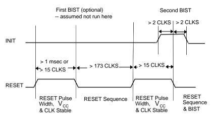
The first RESET pulse is used to ensure that all logic used in the BIST test is correctly initialized; optionally, INIT may be driven high to enter BIST at the falling edge of the first RESET. In this case the results of the first BIST should be ignored.
