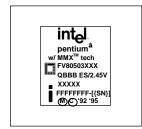
mxB1-Step Pentium® Processor w/ MMX<sup>™</sup> Technology Production PPGA Units:
