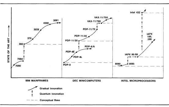
are rare. These few seminal machines instantly elevate the standard for the entire industry, changing the general perception of what a computer is and what it can do. The successful introduction of a quantum machine like the 360 or the PDP-11 inspires a new evolutionary cycle of derivation (and imitation) as the original manufacturer brings out enhanced models, and competitors incorporate the new concepts into their own products.
