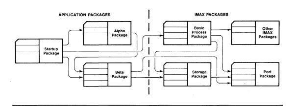
Figure 13. iMAX Package-based Organization germane to the application need be configured. No memory space or processor time is consumed by unneeded facilities. (Naturally, some iMAX packages use each other, so selection of one may implicitly select another.) Furthermore, users may add packages to iMAX, and, within limits, may also replace packages with equivalent local implementations. In sum, iMAX's packagebased organization makes it remarkably adaptable to differing local needs.
