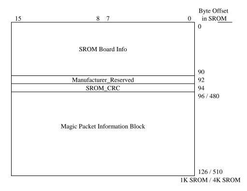
NOTE: Magic Packet information block is supported only by the 21143 Rev 2.0 and above and by the 21145. The 21145 does not support the SecureON password though.
