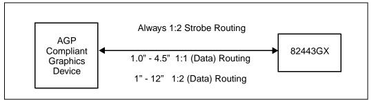
For trace lengths that are between 1.0 inch and 4.5 inches, a 1:1 trace spacing is recommended for data lines. The strobe requires a 1:2 trace spacing. This is for designs that require less than 4.5 inches between the AGP device and the AGP target.
