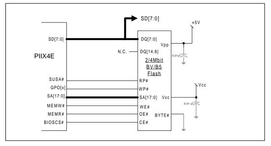
Figure 3-7. Interfacing Intel's Flash with PIIX4E in Desktop
