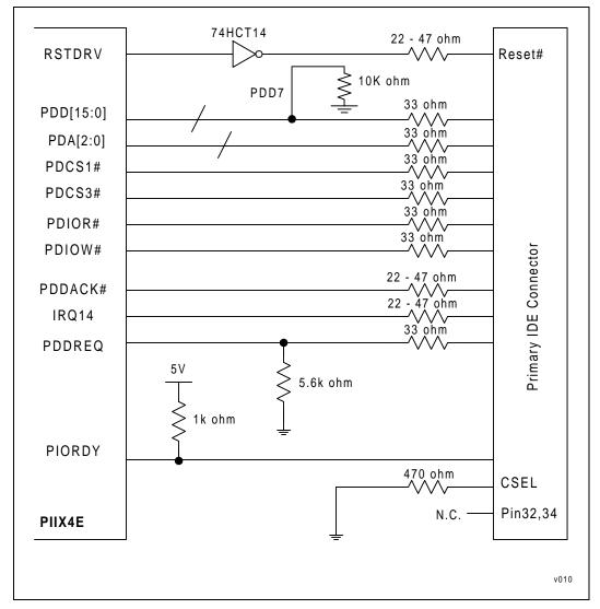
RESET comes from the PIIX4E RSTDRV signal through a Schmitt trigger
