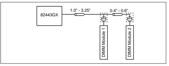
Figure 2-23. Motherboard Model—DQM\_A[1,5], 4 DIMMs
