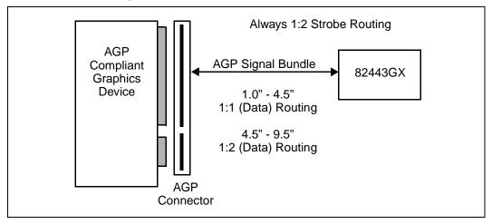
For trace lengths that are between 1.0 inch and 4.5 inches, a 1:1 trace spacing is recommended for data lines. The strobe requires a 1:2 trace spacing. This is for designs that require less than 4.5 inches between the AGP connector and the AGP target.
