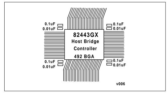
*Note:* There are other discrete components for V<sub>TT</sub>, GTL Ref Voltages that must be also considered when routing around the 82443GX.
