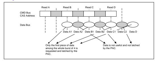
To achieve the burst rate of 1111 during the above scenario, the memory controller needs to support single clock command mode. The output of each command interrupts the ongoing burst or begins at the end of 1st data cycle. With the support of single clock command mode, the timing is shown in Figure 4-4.
