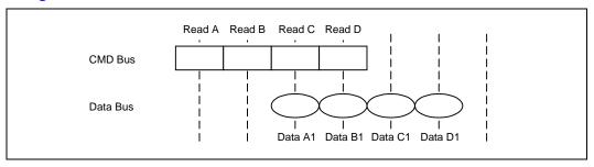
Note that the support of SDRAM single clock command mode is an advanced feature for Intel<sup>®</sup> 440EX AGPset systems on a 3 DIMM design. During a burst pattern of 4 pieces of 64-bit data, if at least the first 2 pieces of data are needed, a Intel<sup>®</sup> 440EX AGPset system can still achieve a burst rate of x111 for SDRAM operation without supporting or enabling single clock command mode.
