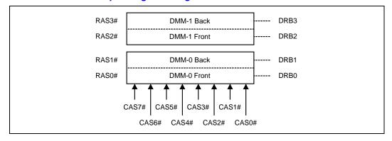
The following 2 examples describe how the DRB Registers are programmed for cases of single-sided and double-sided DIMMs on a motherboard with 4 DIMM sockets.
