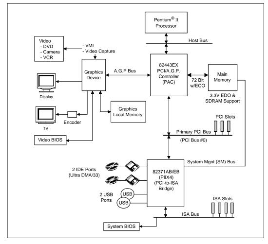
Figure 1-1. Intel® 440EX System Block Diagram
