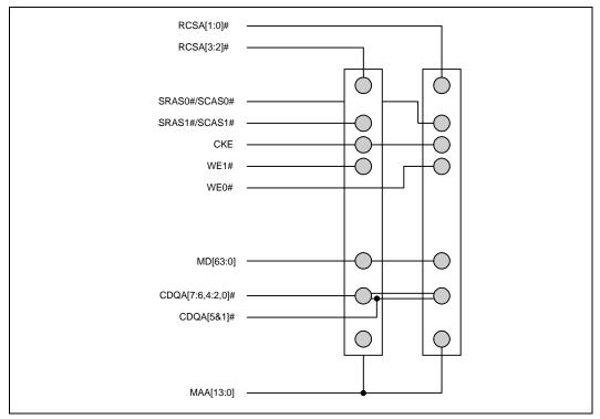
In the 82443EX memory configuration, MAA[13:0] is connected to DIMM sockets 0 and 1. No external buffering is needed on the memory control and address signals.
