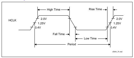
Figure 5-2. 3.3V Clocking Interface
