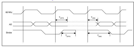
Figure 5-8. AGP 133 Timing Diagram
