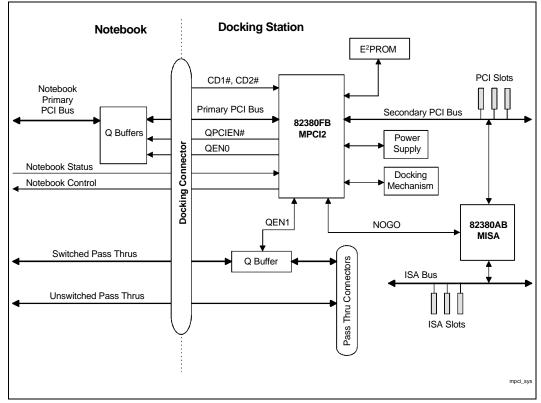
Figure 1. MPCI2 System Block Diagram
