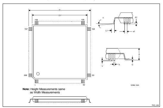
Figure 4. MPCI2 208-Pin SQFP Package
