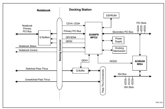
Figure 1. MISA System Block Diagram
