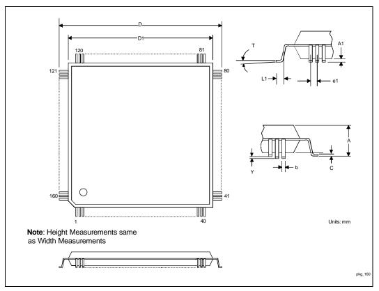
Figure 3. 82380AB 160-Pin MQFP
