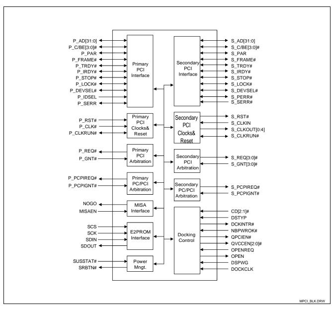
Figure 1. MPCI Block Diagram
