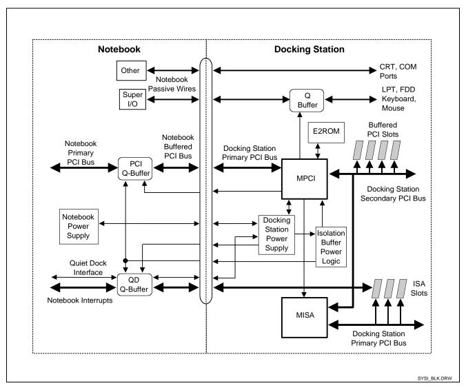
Figure 3. Intel 380AB/PB System Block Diagram
