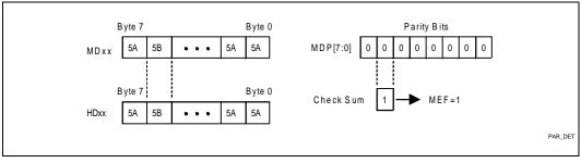
Figure 5. Parity Detection
