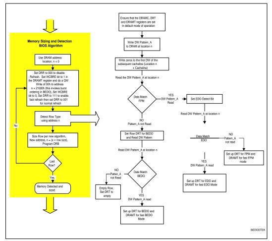
Figure 4. DRAM Auto-Detection Algorithm
