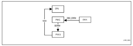
Figure 9. Level 1 SERR# Generation for ECC and Parity
