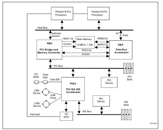
Figure 1. 440FX PCIset System Block Diagram
