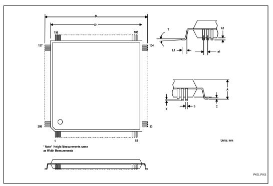
Figure 18. 208 Pin Quad Flat Pack (QFP) Dimensions
