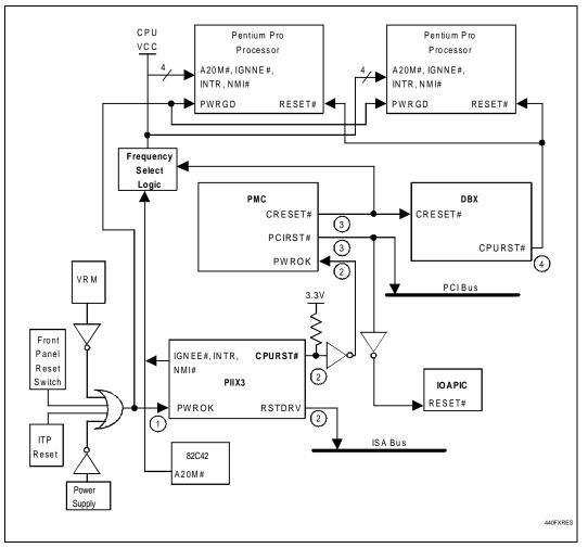
Figure 13. Reset Structure for 440FX PCIset with PIIX3
