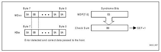
Figure 6. Single Bit Error Detection and Correction (SEC)
