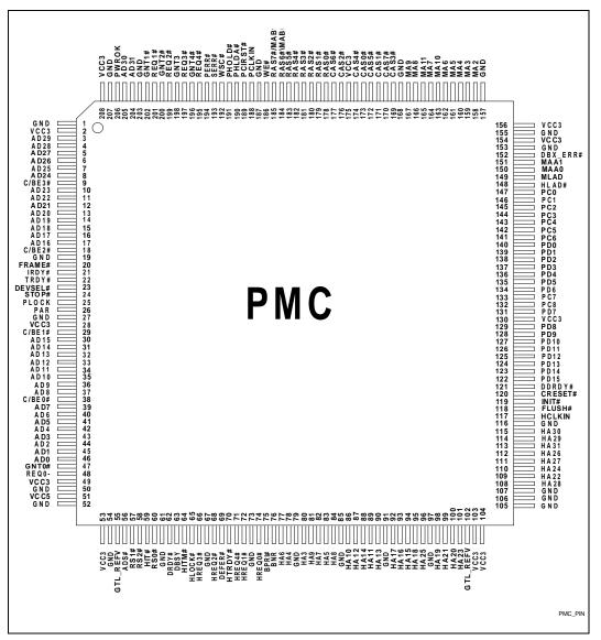
Figure 16. PMC Pinout Diagram
