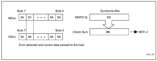
Figure 7. Multiple Bit Error Detection (DED)
