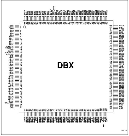
Figure 17. DBX Pinout Diagram
