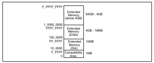
Figure 2. Pentium Pro Processor Memory Address Space.
