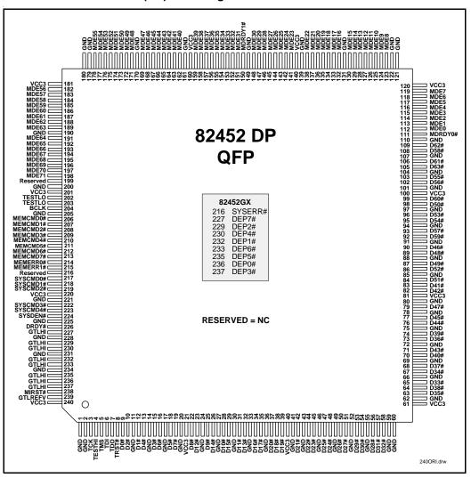
Figure 8. 82452 DP Pin Assignment (240-Pin QFP)
