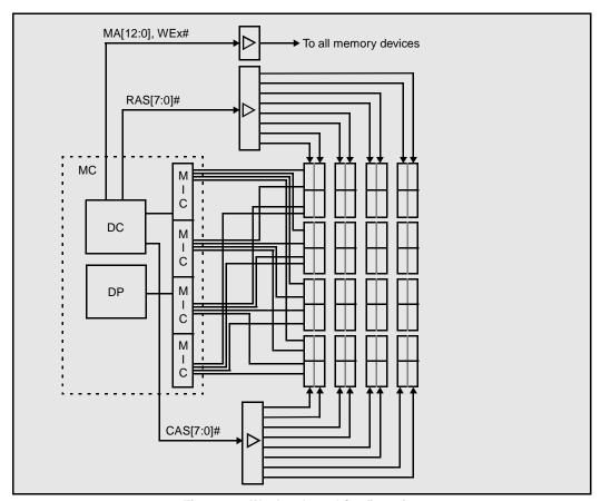
Figure 4. 4-Way Interleaved Configuration
