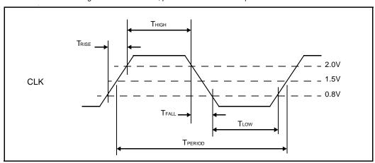
Figure 2. CLock Waveform
