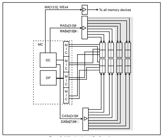
Figure 5. 2-Way Interleaved Configuration
