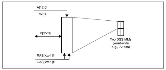
Figure 2. Signal Connections to a Double-Sided SIMM
