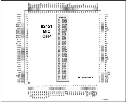
Figure 10. 82451KX/GX MIC Pin Assignment (144-Pin QFP)
