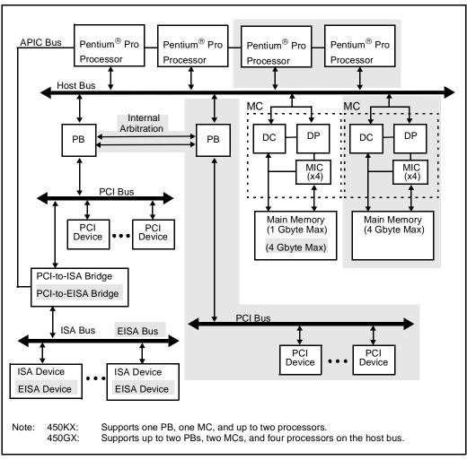
Figure 1. 450KX/GX Simplified System Block Diagram
