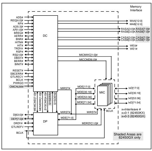
Figure 1. Memory Controller (MC) Simplified Block Diagram
