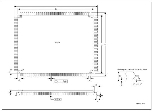
Figure 14. MIC Package Physical Dimensions (144-Pin QFP)
