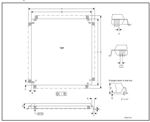
Figure 15. 82454KX/GX PB Package Physical Dimensions (304-Pin QFP)
