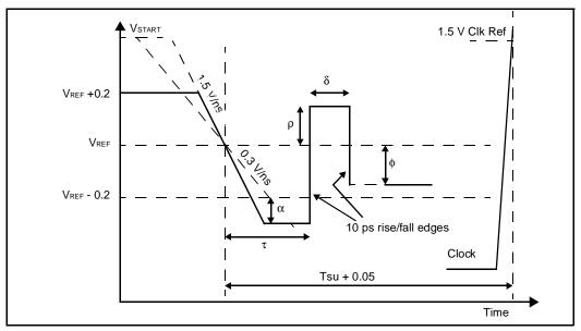
Figure 9. Standard Input Hi-to-Lo Waveform for Characterizing Receiver Ringback Tolerance
