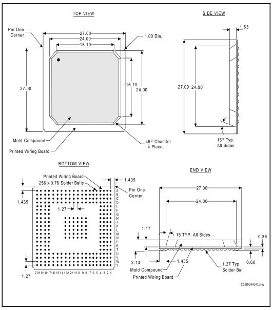
Figure 13. DP Package Dimensions (256 BGA)
