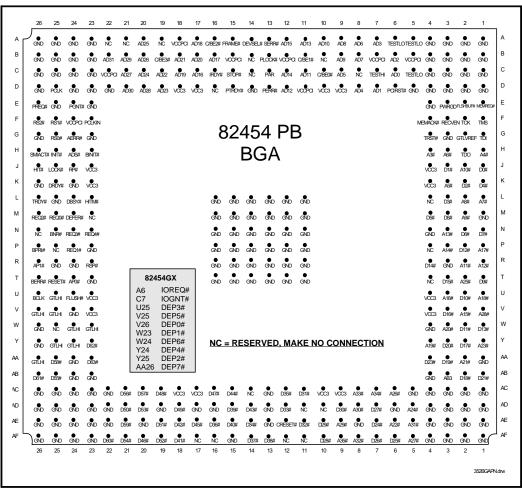
Figure 14. PB Pin Assignment (352 BGA)
