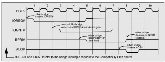
Figure 7. BPRI# Arbitration Timing
