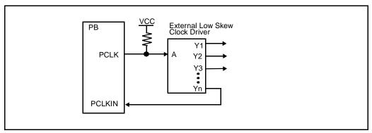
Figure 11. PCI Clock Distribution
