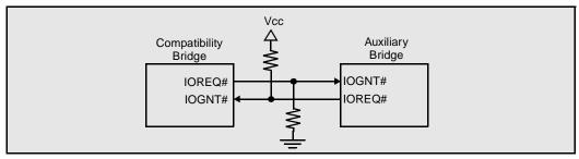
Figure 9. IOGNT# & IOREQ# Pull-Ups/Pull-Downs (Dual Bridge System)
