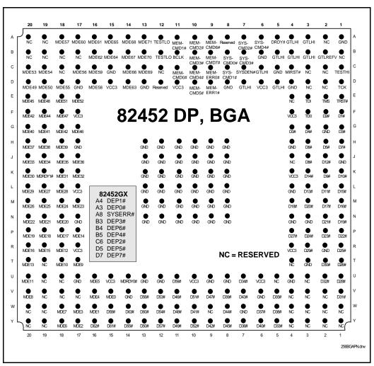
Figure 9. 82452 DP Pin Assignment (256 BGA)
