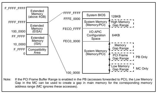
Figure 5. Expanded View of Extended Memory (EISA).
