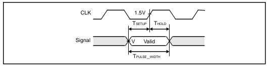
Figure 4. Setup & Hold Timings
