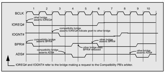
Figure 8. BPRI# Arbitration Overlapped with Bridge Transfer
