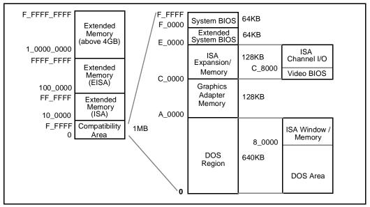
Figure 3. Expanded View of Compatibility Area.
