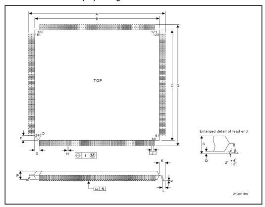
Figure 12. DP Package Physical Dimensions (240-Pin QFP )
