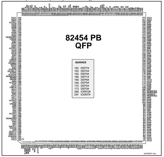
Figure 13. 82454 Pin Assignment (304-Pin QFP)
