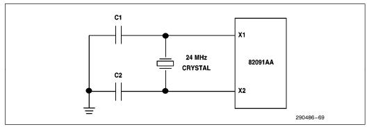
Figure 69. Crystal Connections
