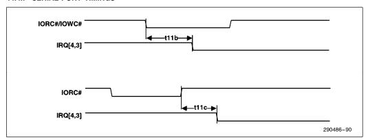
Figure 90. Serial Port Interrupt Timing
