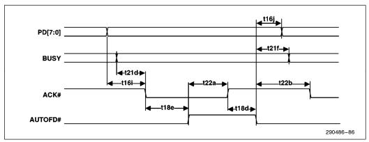
Figure 86. ECP Read Timing (Reverse Direction)
