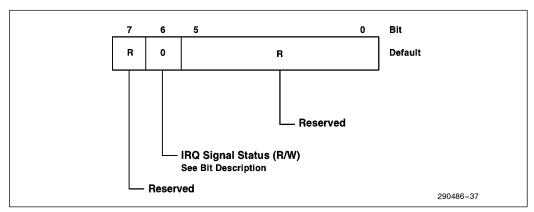
Figure 37. ECP Extended Control Register (ECP Mode)
