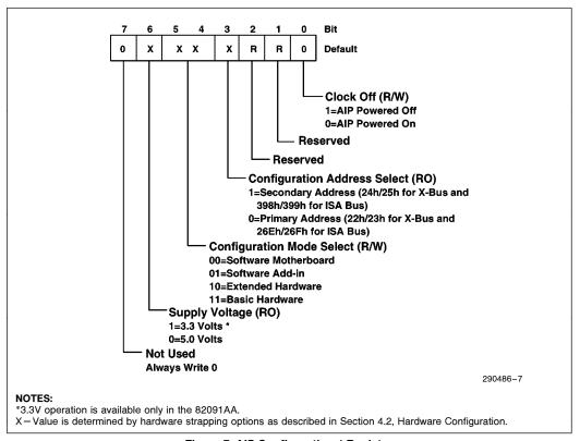
Figure 7. AIP Configuration 1 Register
