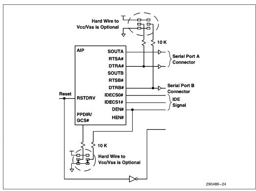
Figure 24. Software Motherboard Hardware Configuration
