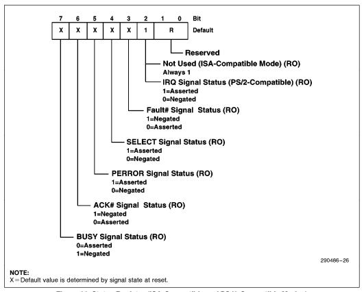
Figure 26. Status Register (ISA-Compatible and PS/2-Compatible Modes)
