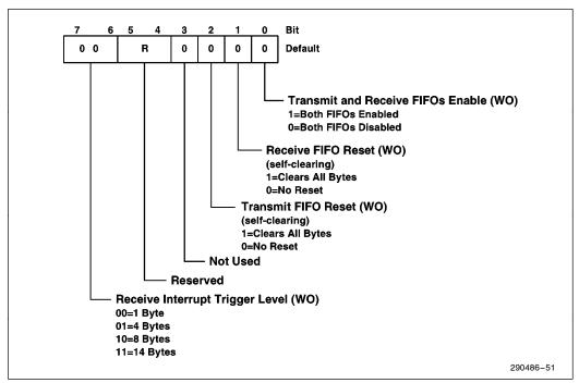
Figure 51. FIFO Control Register
