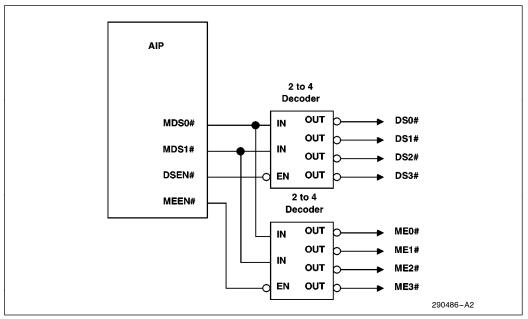
Figure 99. Example External Decoder (Four Drive System)
