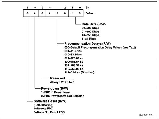
Figure 60. Data Rate Select Register
