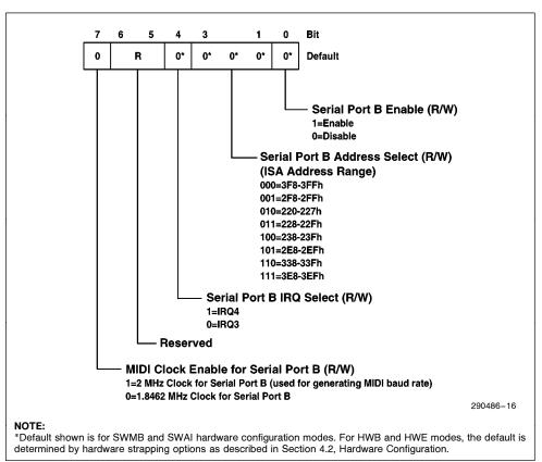
Figure 16. Serial Port B Configuration Register
