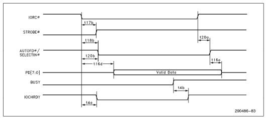
Figure 83. EPP Read Timing
