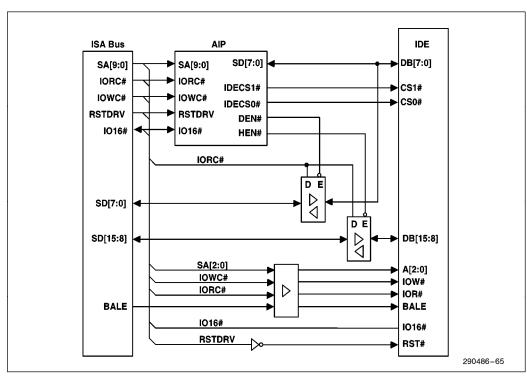
Figure 65. IDE Interface Example (without DMA)
