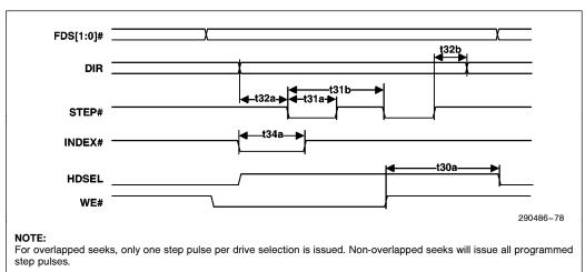
Figure 78. FDC Drive Control/Timing
