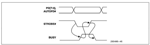
Figure 46. ECP Mode Handshake (Forward Direction)
