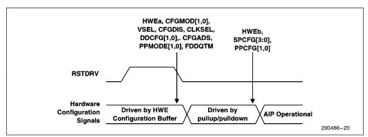
Figure 20. HWE Hardware Configuration Mode Timing
