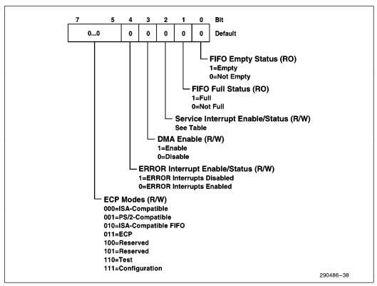
Figure 38. ECP Extended Control Register (ECP Mode)
