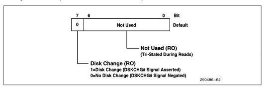
Figure 62. Digital Input Register
