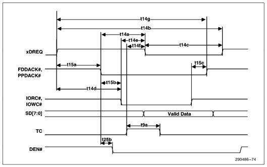
Figure 74. DMA Timing
