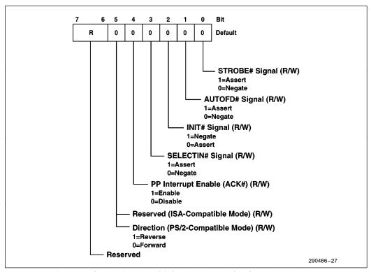
Figure 27. Control Register (ISA-Compatible and PS/2-Compatible Modes)
