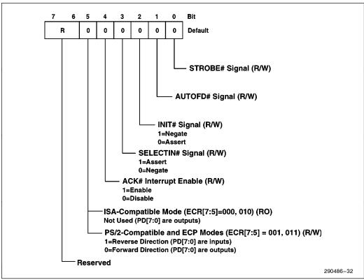
Figure 32. Control Register (ECP Mode)
