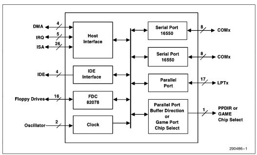
Figure 1. 82091AA Advanced Integrated Peripheral Block Diagram
