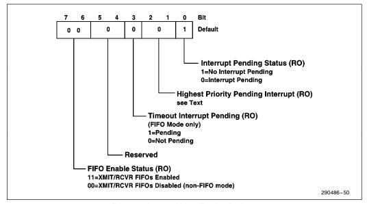
Figure 50. Interrupt Identification Register
