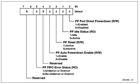
Figure 12. Parallel Port Power Management and Status Register
