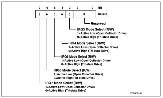
Figure 8. AIP Configuration 2 Register
