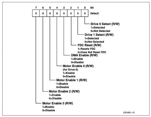
Figure 98. Digital Output Register
