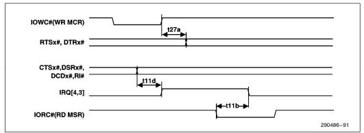
Figure 91. Modem Control Timing
