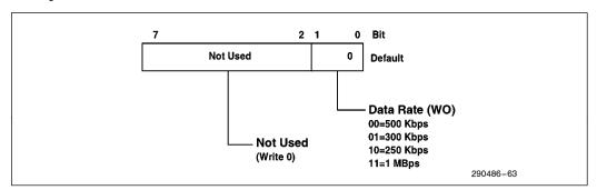
Figure 63. Configuration Control Register
