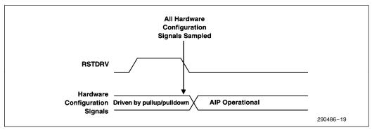
Figure 19. HWB, SWMB, and SWAI Hardware Configuration Mode Timing
