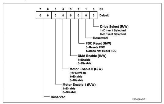
Figure 57. Digital Output Register
