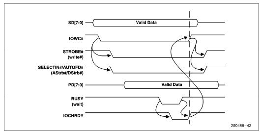
Figure 42. EPP Mode Write Cycle
