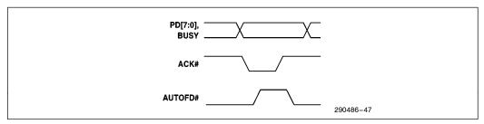
Figure 47. ECP Mode Handshake (Reverse Direction)
