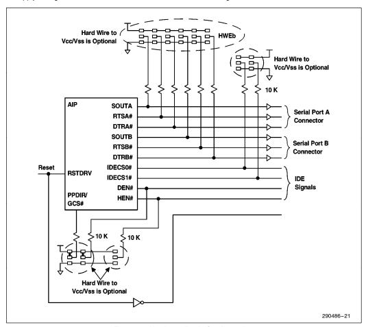
Figure 21. Hardware Basic Configuration
