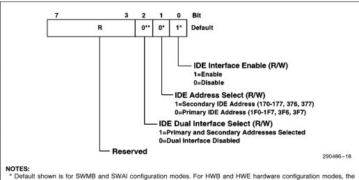
default is determined by hardware strapping options as described in Section 4.2, Hardware Configuration.
