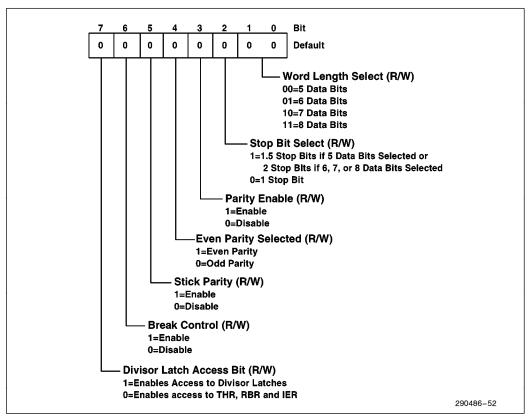
Figure 52. Line Control Register
