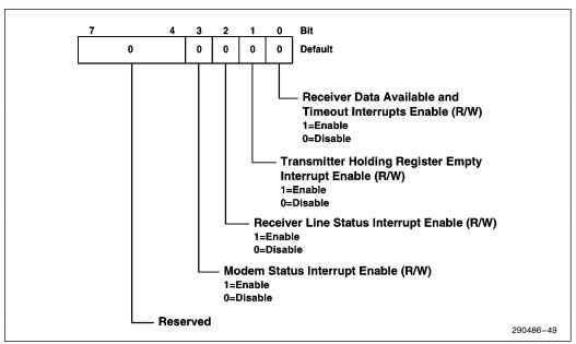
Figure 49. Interrupt Enable Register
