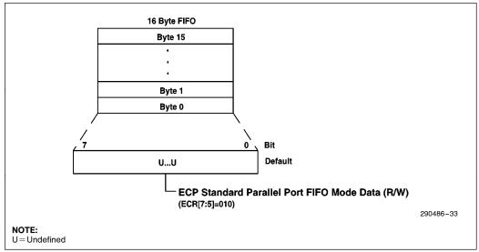
Figure 33. ECP ISA-Compatible Data FIFO
