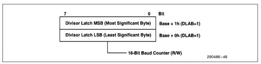
Figure 48. Divisor Latches (LSB and MSB) Registers
