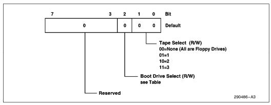
Figure 100. Enhanced Tape Drive Register
