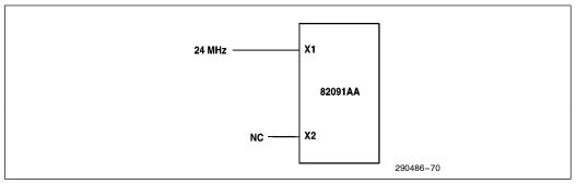
Figure 70. Oscillator Connections
