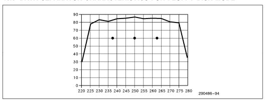
Figure 94. Typical Jitter Tolerance vs Data Rate (Capture Range 250 Kbps)
