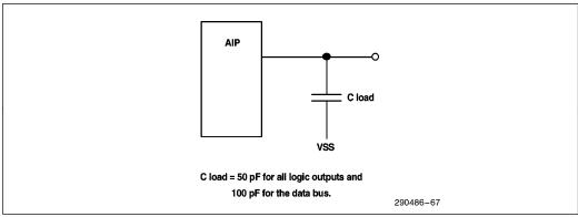
Figure 67. Load Circuit
