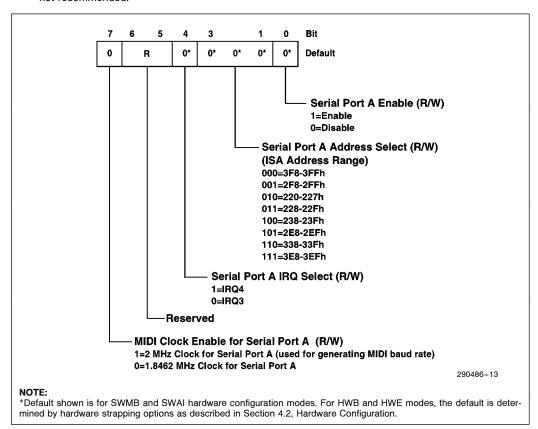
Figure 13. Serial Port A Configuration Register
