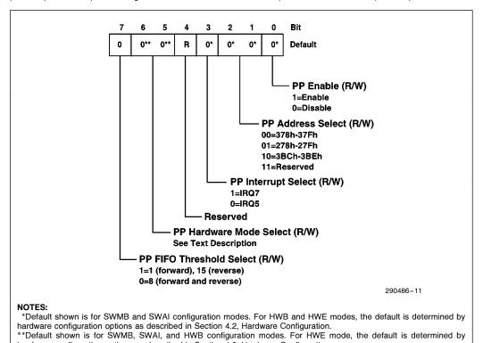
Figure 11. Parallel Port Configuration Register
