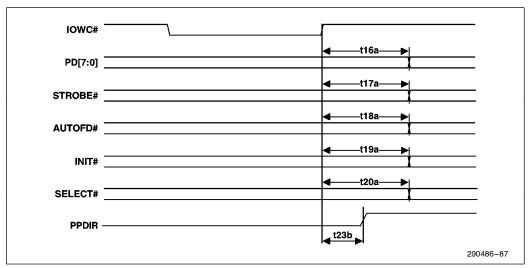
Figure 87. ISA-Compatible Write Timing
