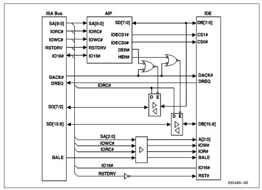
Figure 66. IDE Interface Example (with DMA)
