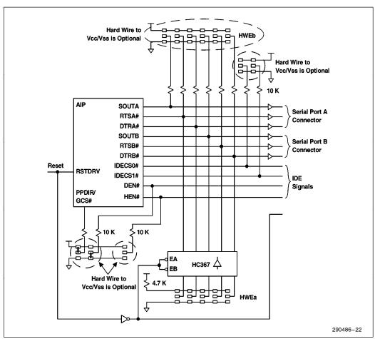
Figure 22. Hardware Extended Configuration
