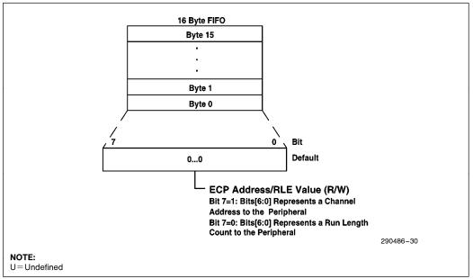
Figure 30. ECP Address/RLE FIFO Register (ECP Mode)
