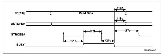
Figure 85. ECP Write Timing (Forward Direction)
