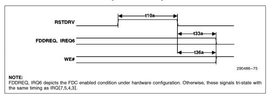
Figure 75. Reset Timing
