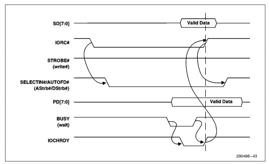
Figure 43. EPP Mode Read Cycle
