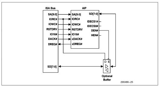
Figure 25. ISA Interface (with Optional Data Buffer)
