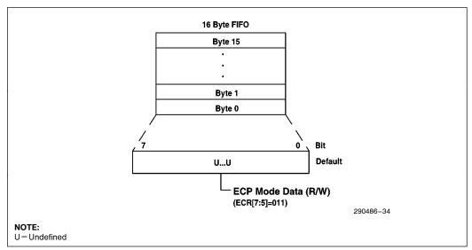
Figure 34. ECP Data FIFO (ECP Mode)
