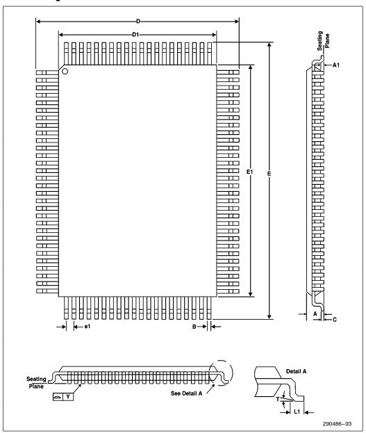
Figure 93. 100-Pin Quad Flat Pack (QFP) Dimensions
