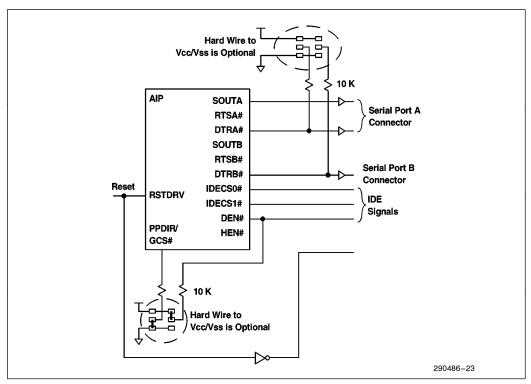
Figure 23. Software Add-In Configuration
