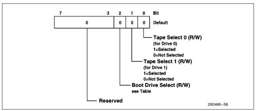
Figure 58. Enhanced Tape Drive Register
