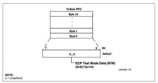
Figure 35. ECP Test FIFO Register (ECP Mode)
