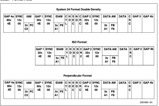
Figure 64. System 34, ISO and Perpendicular Formats
