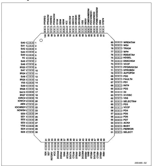
Figure 92. 82091AA Pin Diagram
