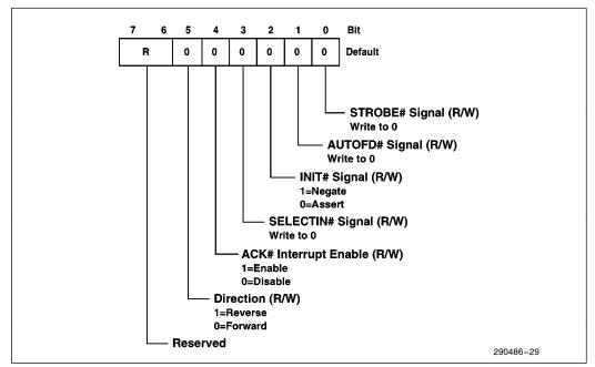
Figure 29. Control Register (EPP Mode)
