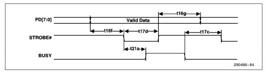
Figure 84. ISA-Compatible FIFO Timing
