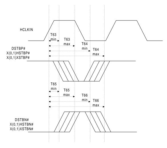
Figure 12-7: Source Synchronous Strobe Timing
