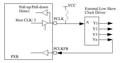
Figure 11-2: PCI Clock Generation and Distribution
