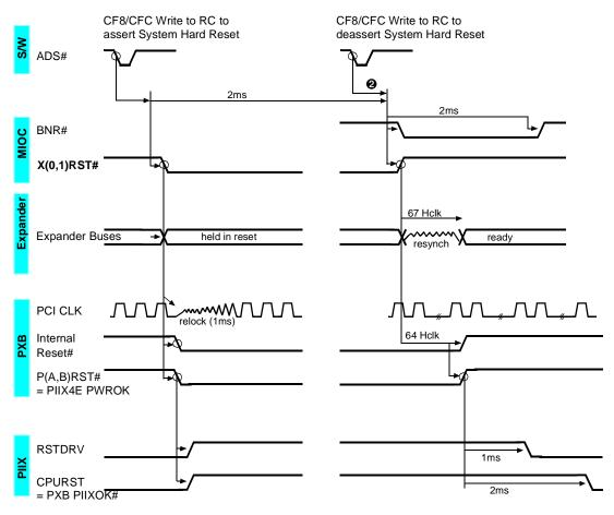
Figure 11-6: Software-Initiated PXB Reset
