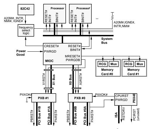
Figure 11-3: Recommended RESET Distribution for Intel<sup>®</sup> 450NX PCIset-Based Systems Including a PIIX4E South Bridge
