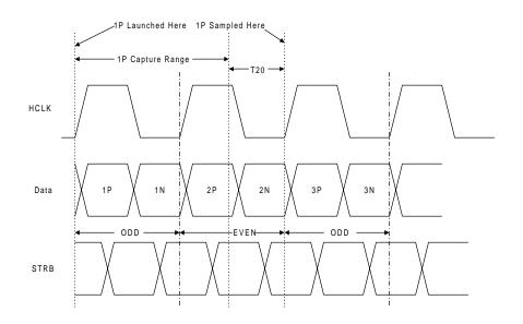
Figure 12-9: Source Synchronous Data Transfer
