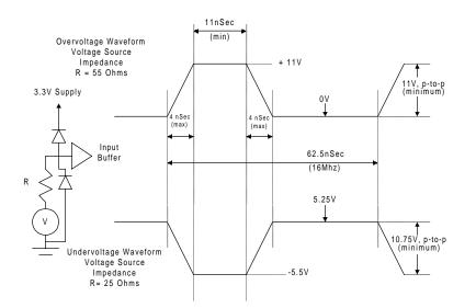
Figure 12-4: Maximum AC Waveforms for 5 V Signaling (PCI Signals)
