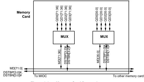
bus. There are two MUX components per board to provide a 72-bit data path from each of four possible interleaved quad-words to the MD bus. This is illustrated in Figure 6-3.
