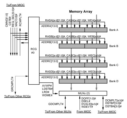
Figure 6-2: Example Showing RCG/MUX Control Signals
