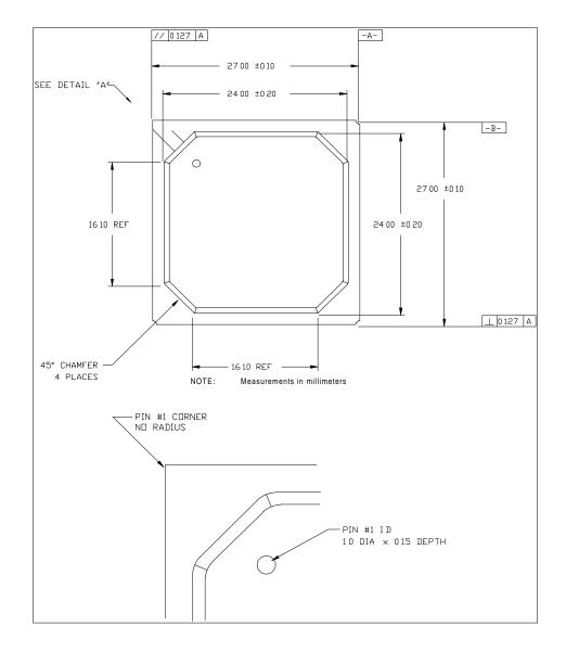
Figure 12-15: 324 BGA Dimension Top View
