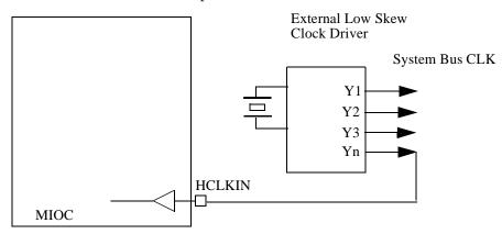
Figure 11-1: Host Clock Generation and Distribution
