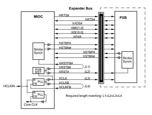
Figure 5-1: Expander Bus Clock Distribution
