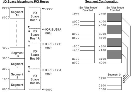
Figure 4-3: I/O Space Address Mapping
