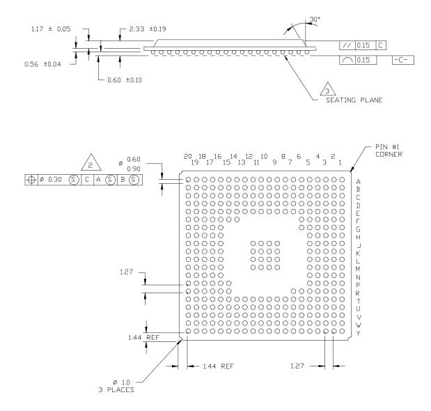
Figure 12-16: 324 BGA Dimensions Bottom View
