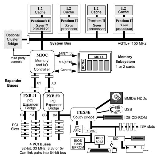
Figure 1-1: Simplified Intel<sup>®</sup> 450NX PCIset System Block Diagram
