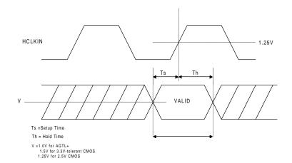
Figure 12-10: Setup and Hold Timings
