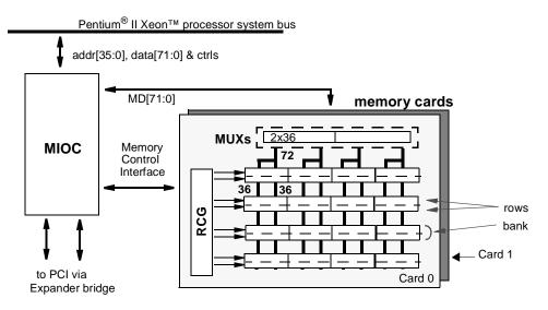
Figure 6-1: Memory Configuration Using 2 Cards
