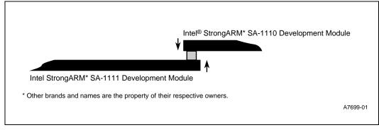
5. To remove the SA-1111 Development Module, evenly pull the modules apart as shown in Figure 2-7.
